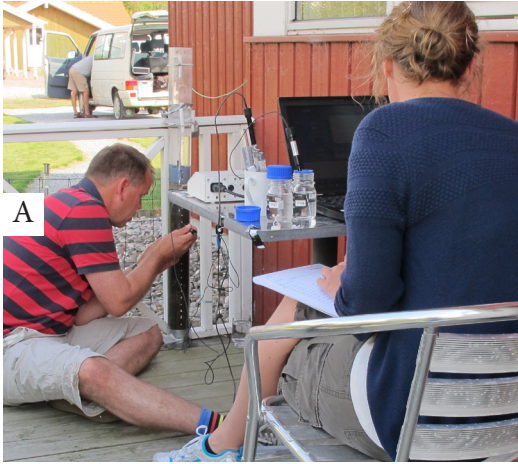
Figure 14. Dr Mikkel Holmen Andersen (Unisense) and Anne Marie Eriksen (National Museum of Denmark) measuring sediment profile parameters in the cores (A). Set up for measuring profiles. The plastic core tubes had silicone filled holes drilled into them every 5 cm, enabling a microsensors to be passed through and the parameters measured (B). Photos National Museum of Denmark.
