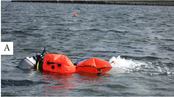
Figure 13. Vibracorer in use as seen from the surface. The lifting bags are designed to both support the vibracorer and make it easier for divers to remove the sediment cores (A). Dr Poul Jensen from AKUT labelling a sediment core (B). Photos National Museum of Denmark.
