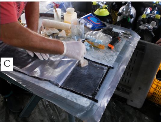
Figure 21. A polyethylene vacuum waterproof bag was first shaped in the form of the artefact to be recovered. The vacuum and waterproof are obtained by adherence of perimetral strips. Before the closure of the strips we had inserted a multilayer composed by Peel Ply tissue (A). Carbon sheet and Peel Ply tissue (B). Inside the bag an epoxy resin was applied over the multilayer (C) and then the bag was closed (D). Photos ISCR.
