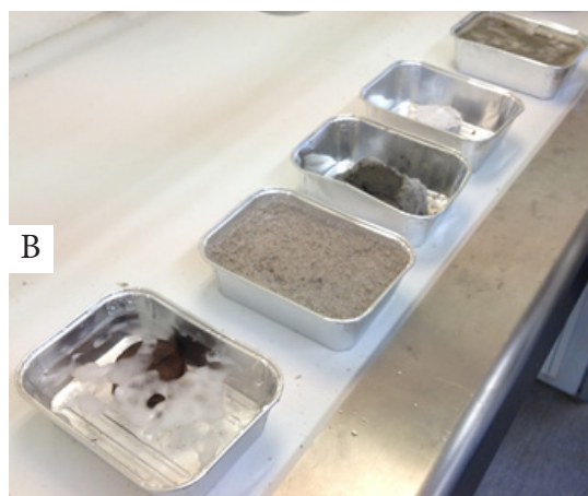
Figure 23. The spear shaft before it was cut into six pieces (A). From the left the wood covered with water is seen next to the wood covered in sand, gyttja, left uncovered and the wood covered with sand and water is seen furthest away (B). Photos National Museum of Denmark.
