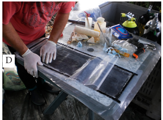
Figure 21. A polyethylene vacuum waterproof bag was first shaped in the form of the artefact to be recovered. The vacuum and waterproof are obtained by adherence of perimetral strips. Before the closure of the strips we had inserted a multilayer composed by Peel Ply tissue (A). Carbon sheet and Peel Ply tissue (B). Inside the bag an epoxy resin was applied over the multilayer (C) and then the bag was closed (D). Photos ISCR.
