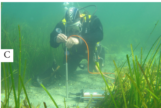
Figure 15. The microsensors with hypodermic needle which is passed into the metal spear and passes through the septum into the sediment (A). End of the spear with the hypodermic needle of the microsensors passing through (B). Inserting the microsensors into the spear (C). Waiting for the sensor to stabilise (D). Photos Viking Ship Museum.
